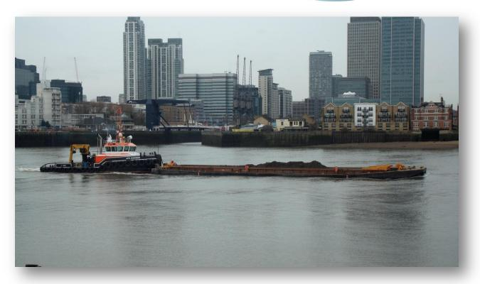
Capacity (Tonnes Dead Weight Cargo Capacity (TDWCC)) 1900 Year of Build 1993 **Operating Area** Cat C, D Waters **Classification/ Certification Society** PLA Registered, Inland Shipping PLA or other No. 28526 **Dimensions: Length, Beam** 56.44m, 11.40m **Light Draught** 0.8m **Loaded Draught** 4m
