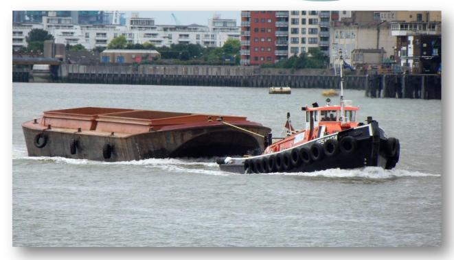
Capacity (Tonnes Dead Weight Cargo Capacity (TDWCC)) 550 **Year of Build** 1970 **Operating Area** Cat C, D Waters **Classification/ Certification Society** PLA Registered, Inland Shipping PLA or other No. **Owners Number: 2054 Dimensions: Length, Beam** 35m, 5.7m **Light Draught** 0.3m **Loaded Draught** 2.7m
