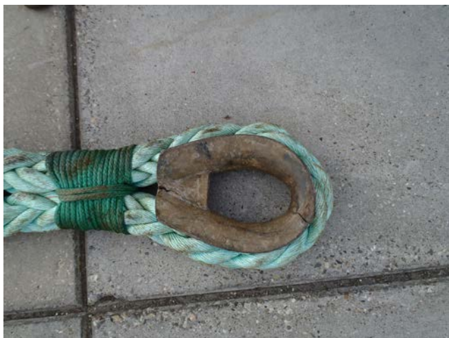
Inspected and rejected due to damaged timble
