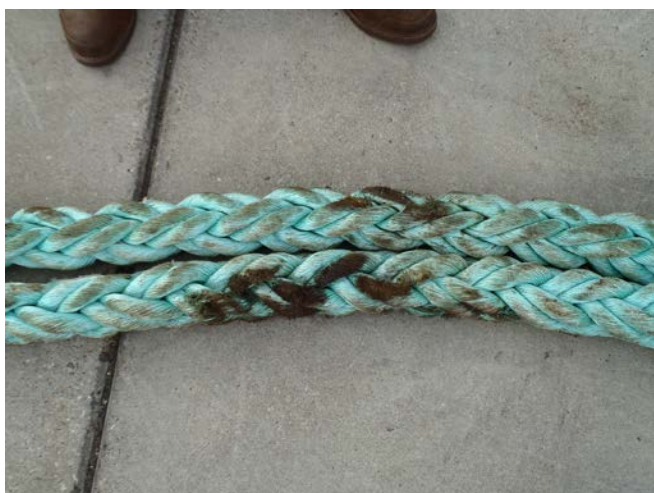
Inspected and rejected due to damage to strands
